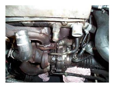
With all that gubbins out of the way simply remove the 2 bolts and one nut holding on the heat shield and take it off.
