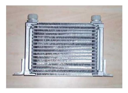
I failed miserably despite the use of releasing oil and a blowtorch, still managed to split the cooler trying to undo the pipes. Above is the new cooler - these are at times impossible to get hold of and I suggest you make sure new ones are available before you get started! It's also worth checking the tightness of the cooler hoses against the cooler after a few weeks.
