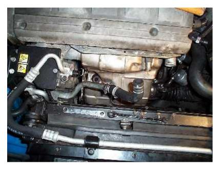
Now, you need to disconnect the second coolant hose and remove the oxygen sensor (lambda probe). To do this you'll need a special 22mm socket which has a cutout in the side for the wiring to pass through. Simply unclip the wiring loom and unscrew the sensor.
