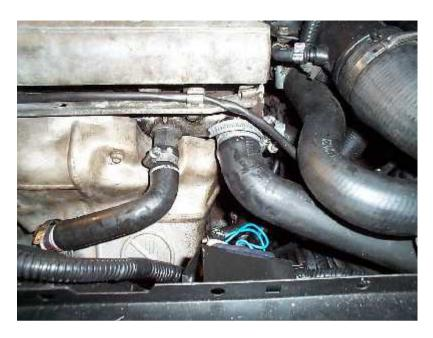
To remove the oil pipes you'll also need to remove the exhaust manifold heat shield as it gets in the way. Remove the coolant hose on the left and drain the system, you can also remove the one on the right to improve access.
