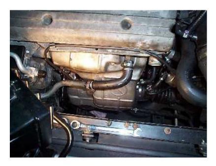
Next, remove the radiator fans to allow enough room to manoeuvre the cover out. The fans are held on with 4 self tapping screws, one of which is accessed from underneath. Disconnect the wiring loom and move it out of the way.
