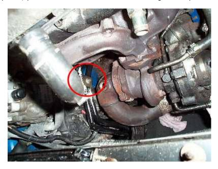
This shows the manifold cover from above with the right hand coolant hose disconnected.
