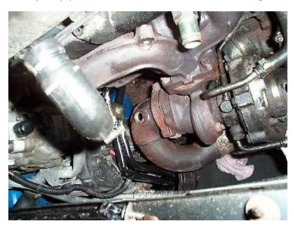
In this photo you can see the oil cooler pipes to the left of the oxygen sensor hole. You can also see a small bracket held on by a 10mm bolt, remove this bolt and bracket first to ease the pipes removal.
