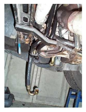
Next, undo the lower support bracket which can be seen in this photo just where the rubber meets the metal pipes.
